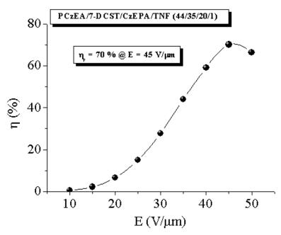
Figure3. High diffraction efficiency for p-polarized beam
