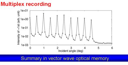
Bragg diffraction with polarization dependence was observed in the polarization gratings. Furthermore, 10 times recording of the orthogonal circular polarization pattern was succeeded. We expect that polarization-sensitive media are applicable to (volume) polarization-sensitive DOEs and optical data storage with polarization.
