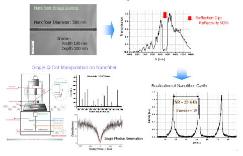
Nanofabrication on Nanofibers: Demonstration Using Focused Ion Beam Method
