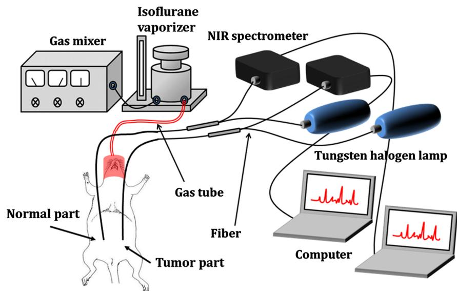
Fig. 1 Experimental setup of NIRS system.
