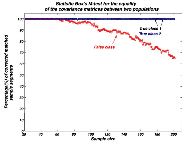
Fig. 7 Experimental results of the Box M-test for the equality of the covariance matrices between the reference and input sample vectors versus the sample size. Two-variate random sample vectors from one section image (well-focused image) were tested.
