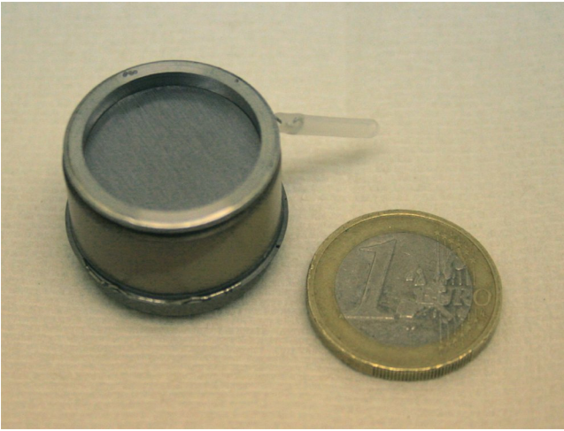
Fig. 10 A bare MXS source, without source holder and LEDs, showing the size, next to a 1€ coin, for comparison. The top of the source shows the beryllium exit window.
