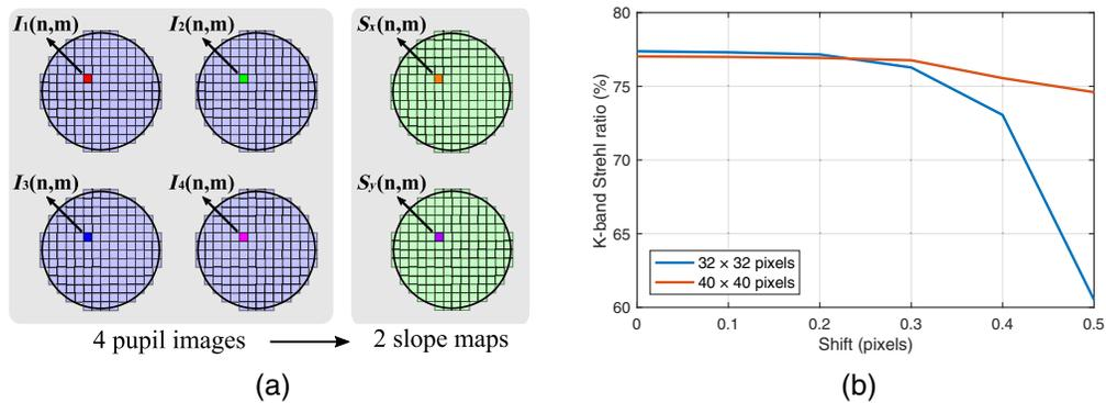
**Fig. 5** Wavefront sampling with a PyWFS: (a) illustration of the pixelation of the PyWFS pupil images and their associated slopes and (b) simulated performance versus fractional pupil shift for the Keck PyWFS with a  $32 \times 32$  DM and different wavefront samplings.
