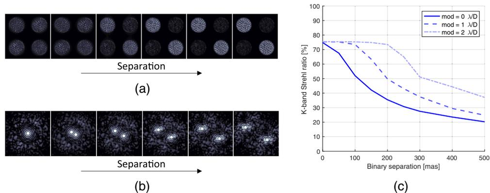
**Fig. 18** Results of simulations of PyWFS behavior in closed loop with equal flux binaries of varying separation: (a) PyWFS images (H-band,  $2\frac{\lambda}{D}$  modulation) for increasing binary separation, (b) focal plane images (H-band) for increasing separation, and (c) Strehl ratio versus binary separation.
