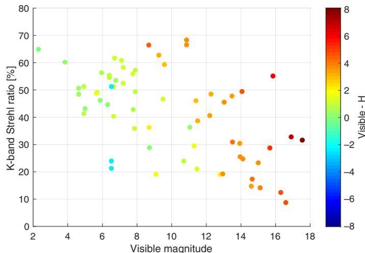
**Fig. 13** Performance of the Keck PyWFS (K-band Strehl ratio) versus visible magnitude. The data points are colored according to the difference between the visible and H-band magnitudes of observed star.
