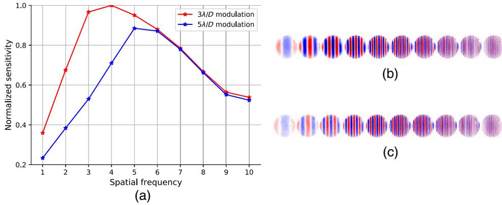
**Fig. 8** Response of the Keck PyWFS to different spatial frequencies: (a) measured sensitivity for 3 and  $5\frac{\lambda}{D}$  modulation, example PyWFS signals for (b)  $3\frac{\lambda}{D}$  modulation, and (c)  $5\frac{\lambda}{D}$  modulation.
