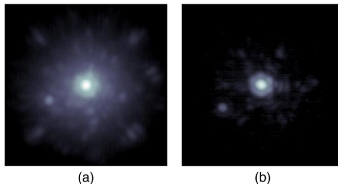
**Fig. 14** K-band images of the system WISEJ0720-0846AB ( $R = 16.9$  and  $H = 9.9$ ) taken with Keck: (a) LGS observation, October 2018,<sup>34</sup> seeing  $\sim 0.5$  arc sec, SR = 22% and (b) PyWFS observation, October 2019, seeing  $\sim 0.6$  arc sec, SR = 46%.
