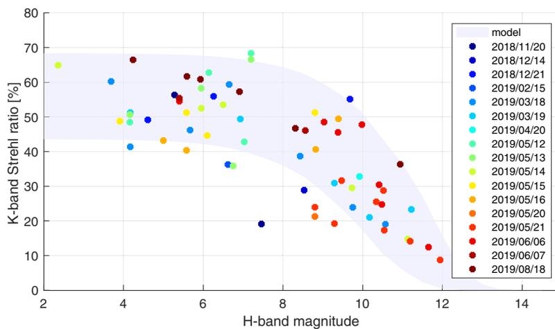
**Fig. 10** Performance history of the Keck PyWFS, in terms of K-band Strehl ratio versus H-band magnitude. Here the color of the data points refer to the date of the measurement: blue points refer to older measurements and red to more recent performance data.
