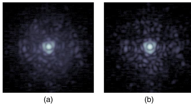
**Fig. 16** K-band images obtained using the Keck PyWFS without modulation, using different control matrices: (a) calibrated for no modulation, SR = 44% and (b) calibrated for  $1\frac{\lambda}{D}$  modulation, SR = 55%. Data taken on August 19, 2019 UT.
