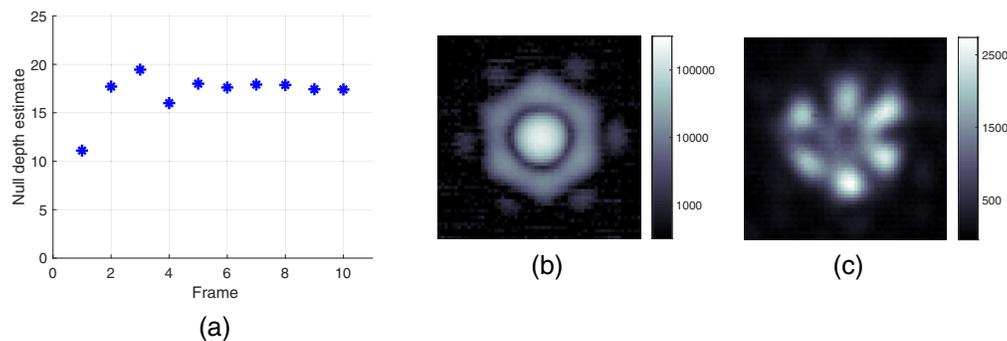
**Fig. 19** Data from one of the best QACITS sequences using NIRC2's L-band vortex coronagraph on Keck II with the PyWFS: (a) estimated null depth over a sequence of 10 images, (b) reference PSF image taken off-axis, and (c) a single science image with the star centred on the vortex. These data were recorded during on-sky operation on June 8, 2019 UT.
