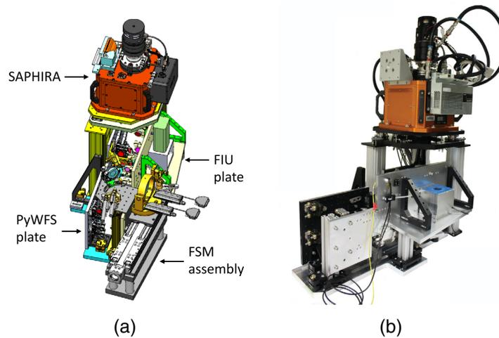
**Fig. 3** (a) CAD drawing of KPIC, including the FSM assembly; PyWFS and FIU plates; and PyWFS (SAPHIRA) camera. (b) KPIC assembled in the laboratory: PyWFS plate (black, background); FIU plate (silver, foreground); and SAPHIRA camera (orange casing).
