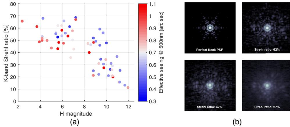
**Fig. 11** On-sky observations with the Keck PyWFS. (a) K-band Strehl versus H-band magnitude. The data points are colored by the effective seeing, taking into account the airmass of the observation. (b) Examples of different quality NIRC2 K-band images. An image of a perfect Keck PSF is shown in the upper left quadrant.
