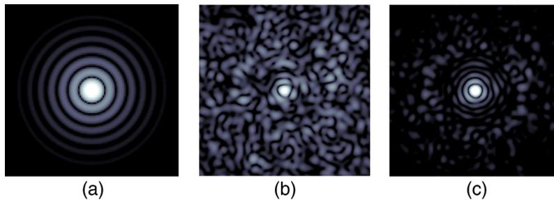
**Fig. 2** Examples of AO corrected and diffraction limited PSFs: (a) a diffraction limited PSF, (b) an AO corrected PSF in the visible (R-band), and (c) an AO corrected PSF in the IR (H-band). The AO corrected examples correspond to the same wavefront error.
