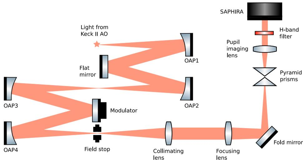
**Fig. 6** Illustration of the layout of the Keck PyWFS optics. The system consists of two OAP relays; a field stop; lenses to provide the correct  $f$ -ratio and WFS sampling for the WFS; and two roof-top prisms to act as the four-sided pyramid prism. A filter within the PyWFS transmits only H-band light and the SAPHIRA detector is used to image the WFS signal.
