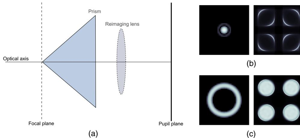
**Fig. 1** (a) Illustration of a PyWFS. The prism angle is exaggerated here for illustrative purposes, but typically have values  $\sim 1$  deg. (b) Focal plane (left) and pupil plane (right) images for a non-modulated PyWFS. (c) Focal plane (left) and pupil plane (right) images for a  $4\frac{\lambda}{D}$  modulated PyWFS.
