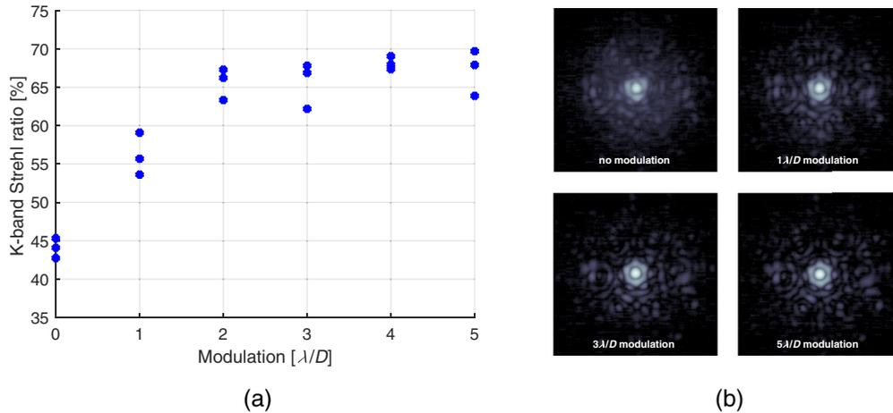
**Fig. 15** The impact of modulation on the performance of the Keck IR PyWFS: (a) K-band Strehl ratio versus modulation radius and (b) K-band images at different modulations. Data taken during on-sky operation on August 19, 2019 UT.
