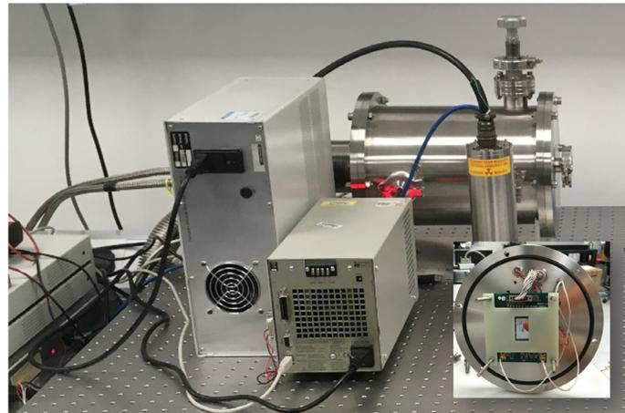
**Fig. 8** The CEI test camera utilizes a 1 MHz XCam XCU-A programmable controller coupled to a custom vacuum cryostat. The headboard and CCD, cooled by a Polycold Cryotiger to  $-105^{\circ}\text{C}$ , is shown in the inset. An x-ray source is incorporated inside the vacuum for use in charge transfer calibration.
