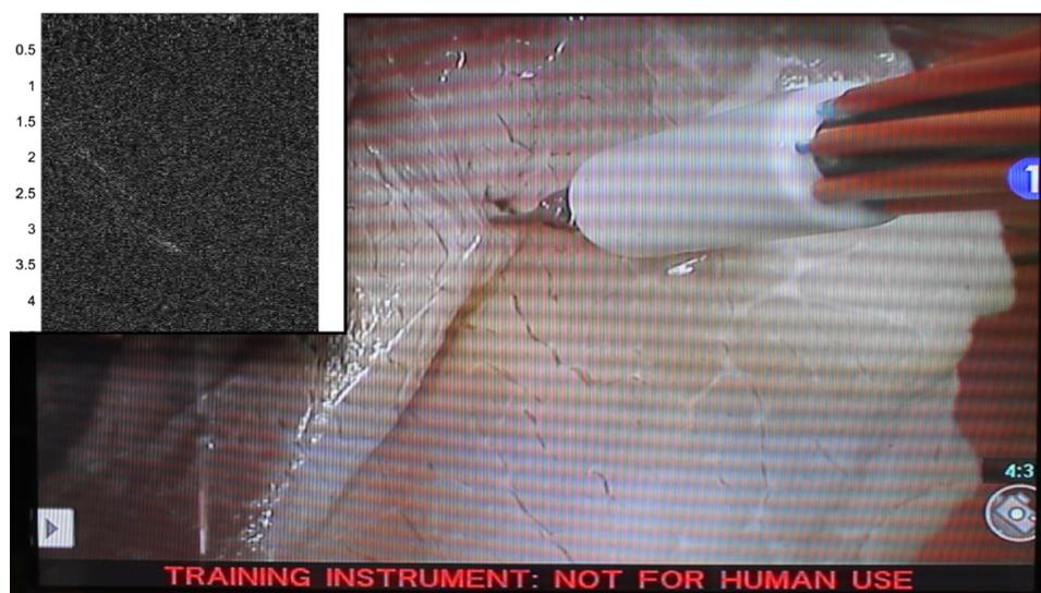
**Fig. 5** Still frame of video showing the sweeping motion of the da Vinci® scissor tool, surrounded by our custom light delivery system. The inset in this video shows the simultaneously acquired photoacoustic images that correspond to the tool sweeping motion (Video 1, MPEG, 6.6 MB [URL: <https://doi.org/10.1117/1.JMI.5.2.021213.1>]).
