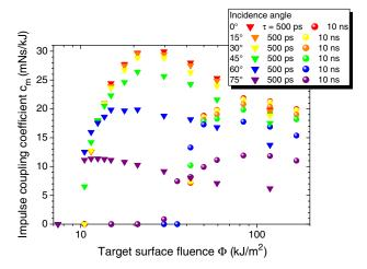
**Fig. 1** Fluence-dependency of the momentum coupling coefficient  $c_m$  in laser ablation of aluminum at  $\lambda=1064$  nm for circular polarized light for two different pulse lengths  $\tau=500$  ps and 10 ns, respectively. Results from simulations with the hydrodynamic code Polly-2T.
