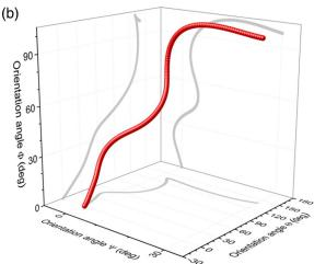
**Fig. 6** Trajectory of (a) position and (b) orientation of pliers under repetitive laser irradiation without tracking. Laser parameters:  $E_L = 1.1$  kJ,  $f_{\rm rep} = 200$  Hz. Operation times out after 0.66 seconds due to the lateral motion of the target. Grey lines indicate the projections of the trajectory in the respective coordinate planes.
