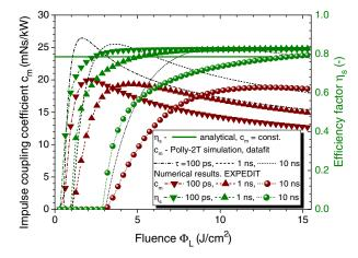
**Fig. 3** Impulse coupling coefficient and efficiency factor  $\eta_s$  for laserablative momentum coupling for a cylindrical target using fit results for  $c_m(\Phi_T)$  for various pulselengths, 100 ps, 1 ns, and 10 ns, from hydrodynamic simulations with Polly-2T. Numerical results with EXPEDIT are compared with the analytical solution from Ref. 10, which is indicated by the horizontal line.
