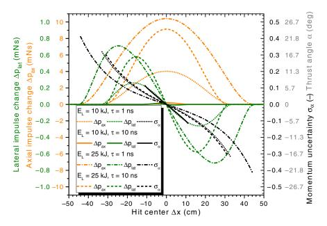
**Fig. 4** Momentum components  $p_{\rm ax}$ ,  $p_{\rm lat}$ , thrust angle  $\alpha$ , and momentum uncertainty  $\sigma_a$  for laser-ablative momentum generation on a solid aluminum sphere with d=10 cm diameter by a laser pulse with a spot diameter of  $d_{\rm FWHM}=50$  cm for various laser pulse energies  $E_L$  and pulselengths  $\tau$ .
