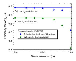
**Fig. 2** Shape-related efficiency  $\eta_s$  of laser-ablative momentum generation for a cylindrical and a spherical target: Numerical results from EXPEDIT in comparison with the theoretical solution following the area-matrix concept<sup>10</sup> indicated by the horizontal lines.
