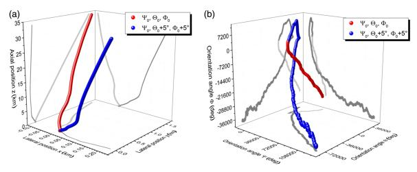
**Fig. 7** Sample trajectories of (a) position and (b) orientation of the pliers with activated tracking for two different initial conditions. For the blue trajectory, a slightly different initial orientation of the target was chosen. Gray lines indicate the projections of the trajectory in the respective coordinate planes and light gray refers to the red trajectory. Laser parameters: see Fig. 6.
