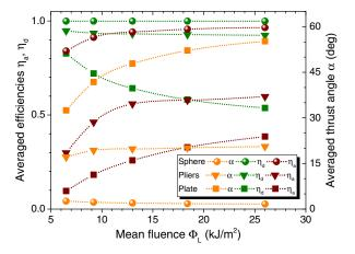
**Fig. 8** Results from Monte-Carlo simulations with EXPEDIT comprising 500,000 different initial positions and orientations of the target giving the averaged figures of merit  $\eta_a$ ,  $\eta_d$  and the thrust angle  $\alpha$  for laser-induced momentum generation. Target geometries: plate (10 cm edge length), pliers (12-cm maximum dimension), and sphere (10-cm diameter). Gaussian laser spot profile with 50-cm diameter (full width half maximum, FWHM).
