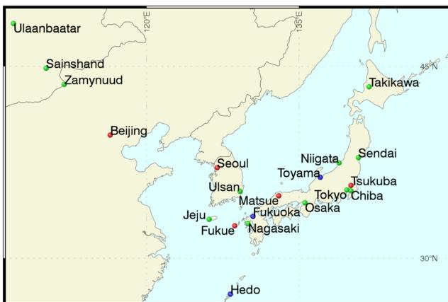
**Fig. 1** Locations of current AD-Net lidar observatories. Green, red, and blue symbols indicate locations of EL, RL, MRL systems, respectively.
