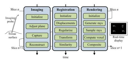
Fig. 5 Flow diagram of the coupled imaging-registration-rendering pipelines.
