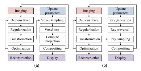
Fig. 3 Pipeline for deformation integrated rendering: (a) object-ordered rendering and (b) image-ordered rendering.
