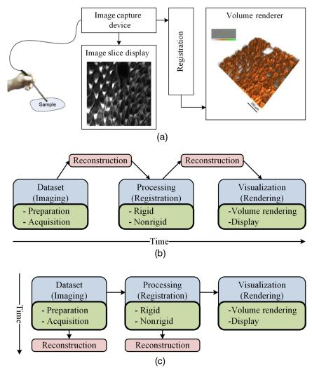
Fig. 2 The imaging pipeline: (a) an imaging procedure, (b) a canonical 3-D medical imaging pipeline, and (c) our proposed pipeline.
