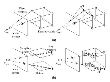
Fig. 4 Nonrigid interpolation for (a) object-ordered rendering: values of origin points are replaced by values from a deformed point, (b) image-ordered rendering: sampling point locations are displaced from deformation. Left: original rendering model; Right: displacement model.
