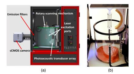
Fig. 2 Illustration of the TriTom imaging system (a) and a picture of the imaging chamber (b).
