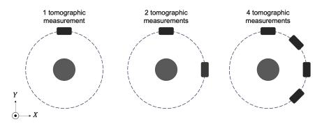
Fig. 3 Top view of the virtual imaging systems collecting 1, 2, or 4 tomographic measurements per imaging frame.
