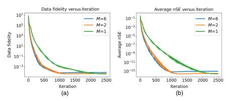
**Fig. 7** Data fidelity versus the iterations (a), and the average nSE versus iterations (b). The plots confirm the correct implementation of the algorithm and illustrate how increasing the number of subsets can accelerate the reduction of the data fidelity term. Additionally, the plots illustrate the similar order-of-magnitude reduction in both data fidelity and average nSE values for every number of subsets  $M \in \{1, 2, 6\}$ .
