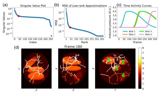
**Fig. 5** (a) Singular value plot of the dynamic numerical phantom, (b) MSE of low-rank approximations, (c) TACs at the center of each ellipsoidal blob, and (d) maximum intensity projection (MIP) images of the 180th object frame of the dynamic phantom (bottom). The ellipsoidal blobs are numbered in the MIP along the z-axis image. The red dot in panels (a) and (b) denotes the index  $R_{max} = 40$  used as a maximum rank constraint in the reconstruction studies.
