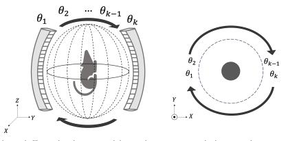
Fig. 1 Schematic illustrating the sequential scanning strategy employing a rotating acoustic probe around the object.
