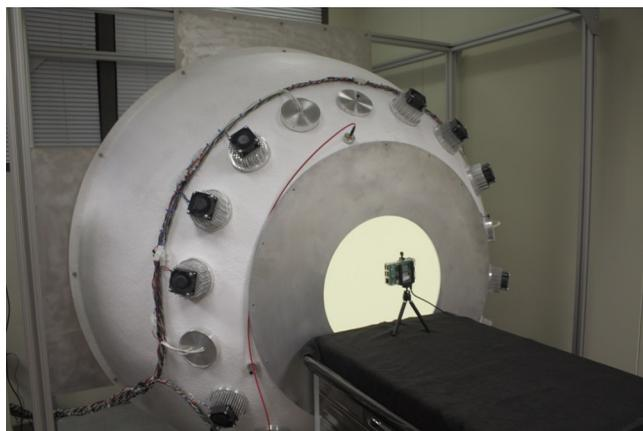
Fig. 5 Raspberry Pi camera acquiring imagery of an I2R integrating sphere lamped with white-light LED sources.
