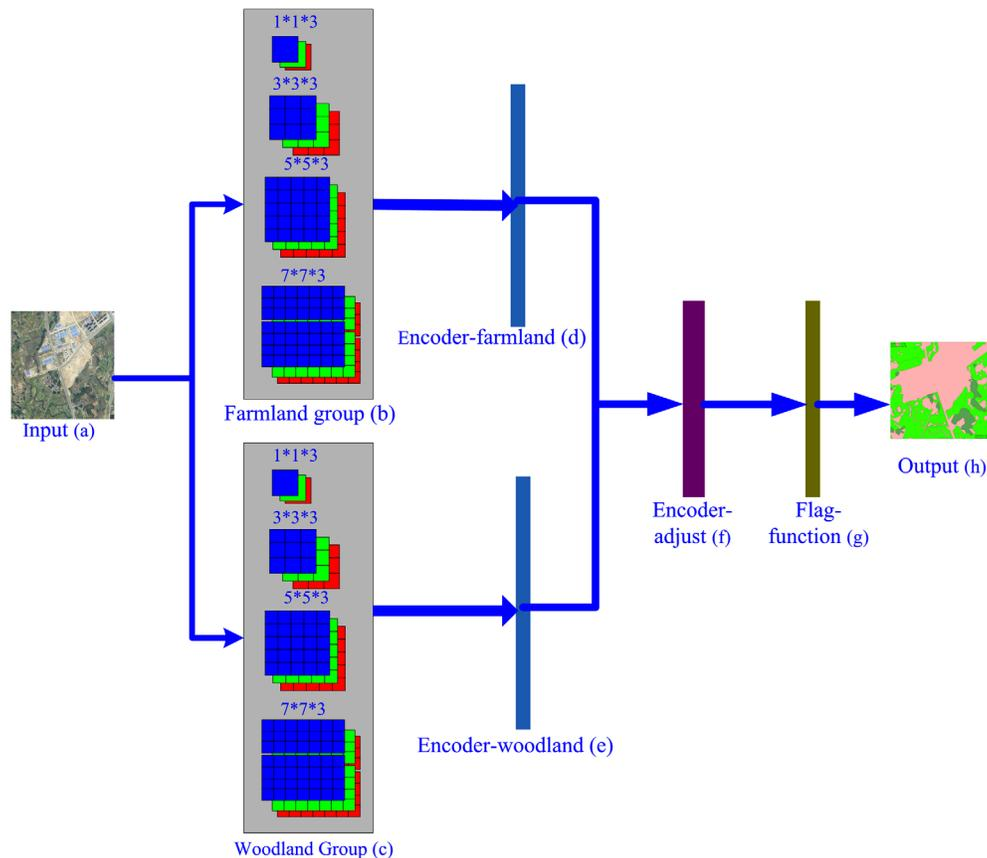
**Fig. 2** The network architecture of CENNs.
