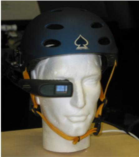
**Fig. 9** Full-color monocular HWD circa 2007, 2 pounds. Outside-in laser head tracking.
