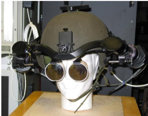
**Fig. 3** Full-color binocular prototype HMD by Microvision circa 2003, 10 pounds.
