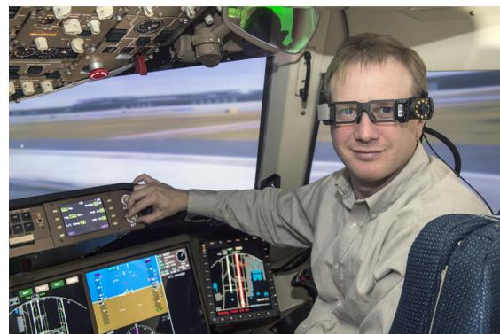
**Fig. 6** Lumus DK-32 display glasses coupled with a prototype head tracker made by Thales Visionix.
