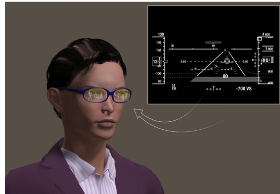
**Fig. 5** Concept picture of a lightweight sunglasses form factor HMD for commercial aviation use.
