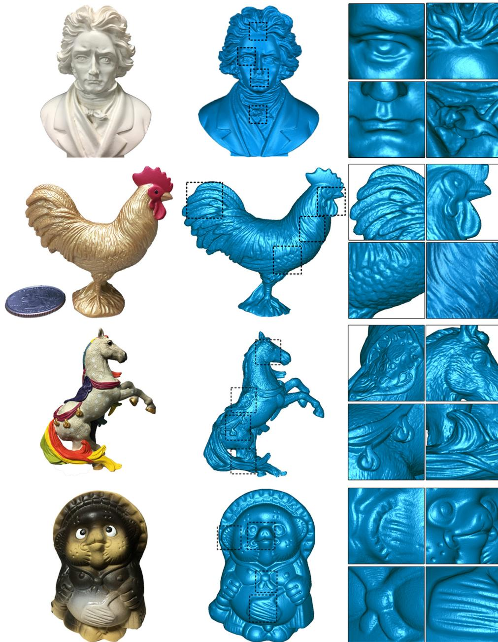
**Fig. 13** Scanning result for various objects, constructed of gypsum, plastic with metal coating, rubber, and earthenware, respectively.
