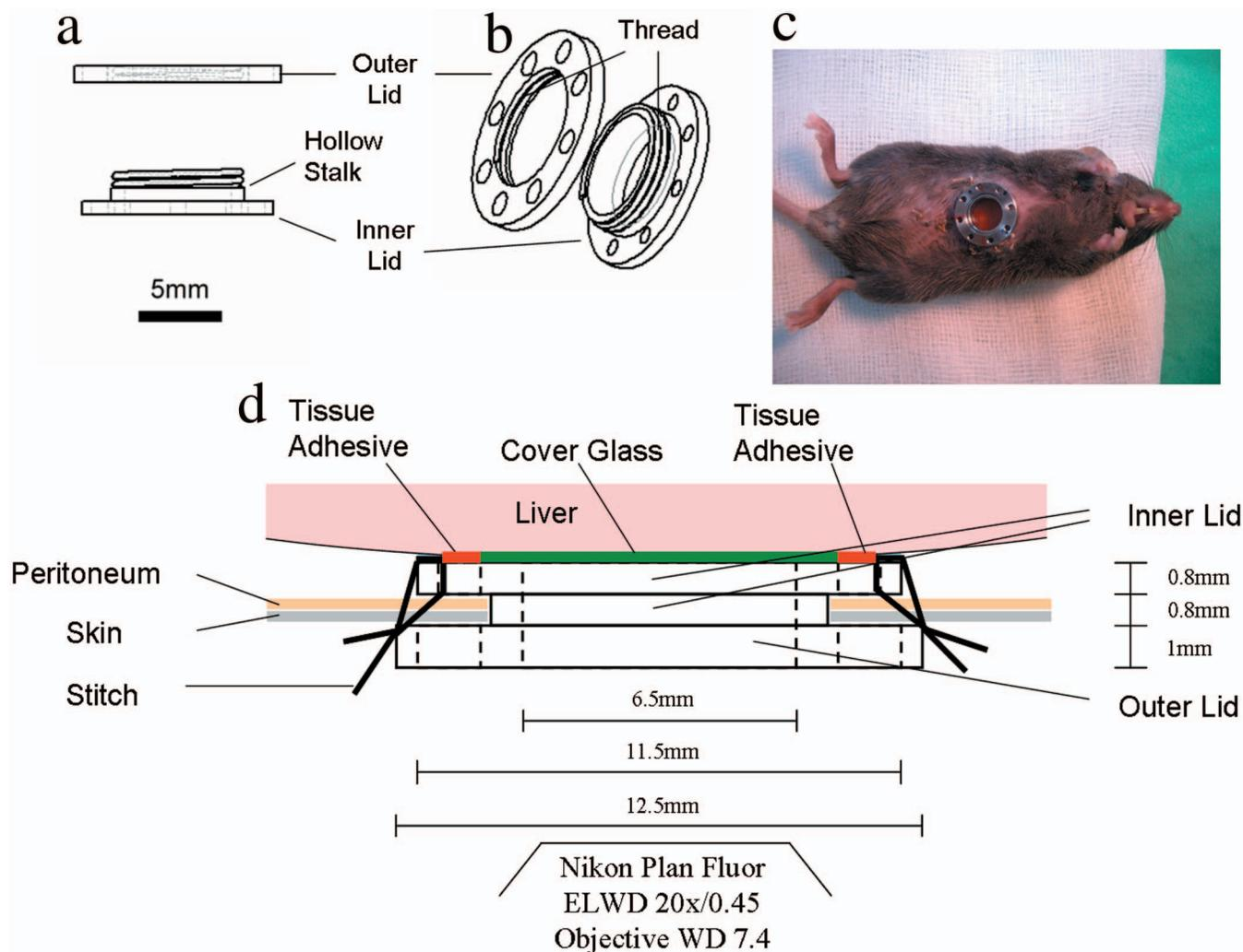
**Fig. 1** Illustrations showing the structure of the hepatic imaging chamber and its anatomic position after installation on the mouse abdominal wall. (a) Horizontal and (b) oblique views of the chamber apparatus. (c) A photograph showing a mouse with the device installed on its upper abdominal wall. (d) A diagram depicting the anatomic relationships of the installed device with skin, peritoneum, and the underlying liver.
