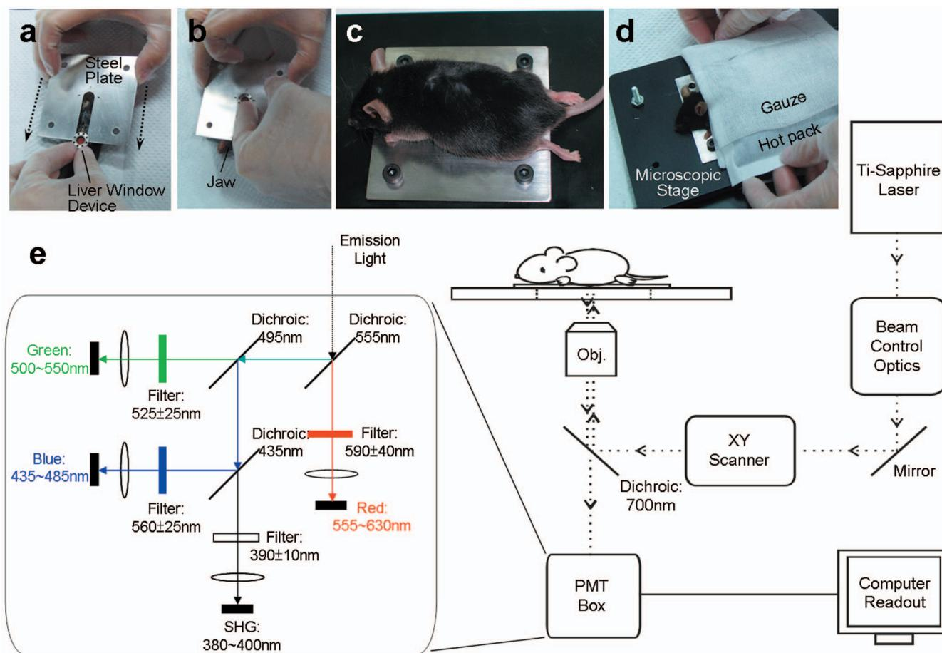
**Fig. 2** Accommodation of the mouse on the microscope stage. Fixing of the mouse with its hepatic imaging chamber into the groove of a steel plate was shown in (a), (b), and (c). (d) Fixing the plate onto the microscope stage by screws. (e) A brief schematic of the imaging light path.
