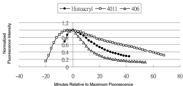
**Fig. 5** Measured normalized fluorescence intensity profiles using the glues of Histoacryl, 4011 (for medical device, Henkel Loctite), and 406 (instant adhesive, Henkel, Loctite).
