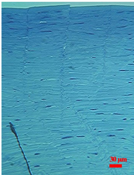
Fig. 6 Histological section of laser incisions in an edematous cornea performed at NA=0.6 with correction of spherical aberrations at depths of 300, 450, and 640 \mu\text{m} , respectively (from left to right).
