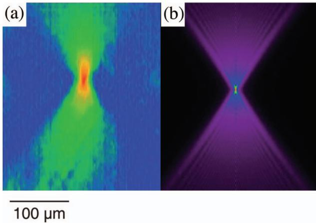
**Fig. 3** Illustration of PSF modeling. (a) The  $x$ - $y$  view of the cone of light from a dendrite. Its intensity distribution is approximately symmetric with respect to the focal plane and the optical axis. (b) Modeled PSF obtained by treating the TLB microscope as if it would be a fluorescent microscope that suffers from no primary aberrations. These assumptions have been verified (Ref. 21). (High resolution image available online only.)
