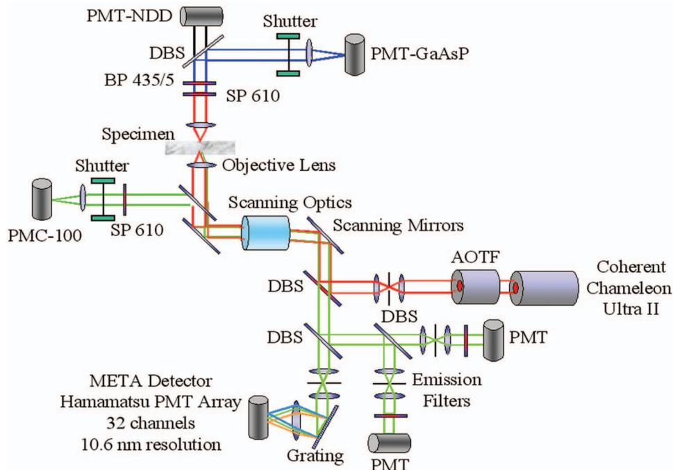
**Fig. 1** Experimental setup. PMT is the photomultiplier tube, NDD is the nondescanned detector, DBS is the dichroic beam splitter, BP is the bandpass filter, SP is the short pass filter, AOTF is the acousto optical tunable filter, and GaAsP is gallium arsenide phosphide.
