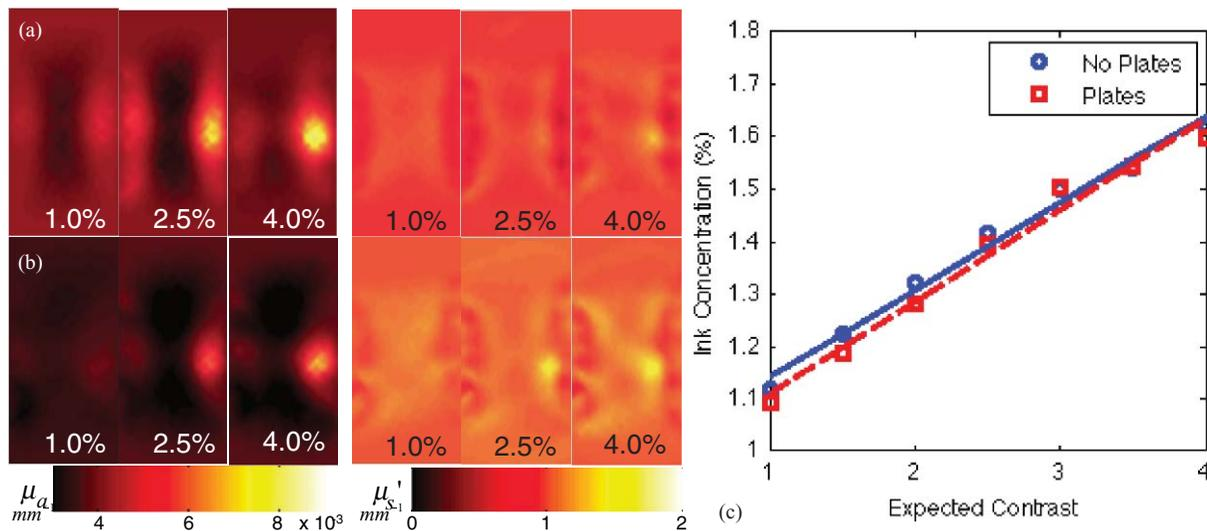
**Fig. 3** Images from phantom experiment showing system linearity with (a) and without (b) faceplates. The left block of images quantify  $\mu_a$  ( $\text{mm}^{-1}$ ) in the domain while the right block shows  $\mu_s'$  ( $\text{mm}^{-1}$ ). The percentage of ink solution concentration used is written on each image. The graph (c) shows results of linearity over different ink solution concentrations with associated linear regression lines.
