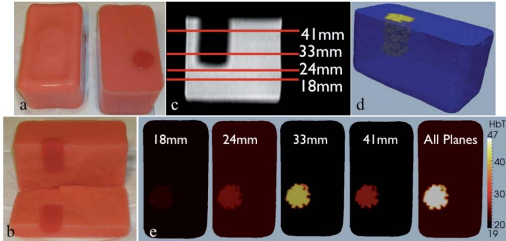
**Fig. 4** Phantoms used (a) and (b) in experiment showing contrast recovery. Axial MR image of inclusion phantom (c) with locations of 4 imaging planes shown and text reporting imaging plane distance from bottom of phantom. 3D representation (d) of reconstruction using all 4 data sets simultaneously, and slices (e) through the inclusion after being reconstructed by individual data sets.
