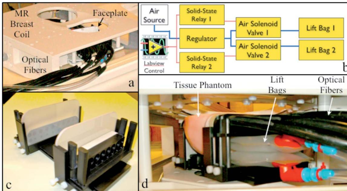
**Fig. 1** MR breast coil with MR-optical breast interface integrated (a) and block diagram of control system used to remotely move fibers (b). Photos of interface (c) showing location of the optical fiber-tissue interface (black circles) and (d) in MR breast coil from side with lift bags, optical fibers, and tissue-simulating phantom.
