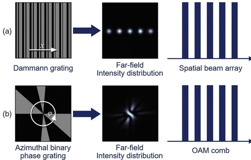
**Fig. 1** Analogy between the Dammann grating and the azimuthal binary phase grating (OAM comb). (a) Dammann grating and spatial beam array. (b) Azimuthal binary phase grating and OAM comb.
