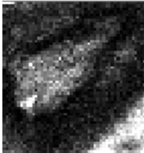
Fig. 4 Pixel purity index (PPI) image. This image was created using the first three MNF bands. The white areas show the pixels selected as those that had the greatest occurrence as extreme, and are, thus potential endmembers.
