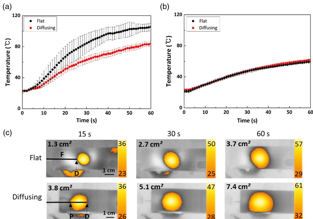
**Fig. 4** Temporal development of temperature in adipose tissue: (a) flat fiber (20 W) and diffusing applicator (20 W), (b) flat fiber (10 W) and diffusing applicator (16 W), and (c) thermal images acquired at various irradiation times (15, 30, and 60 s) with flat fiber (10 W) and diffusing applicator (16 W). Note that the numbers in left upper corners represent the area of temperature distribution (F = fiber, P = proximal end, D = distal end).
