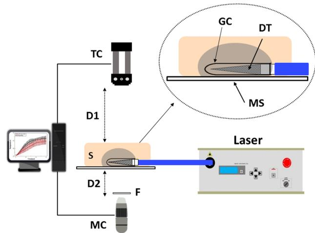
**Fig. 1** Experimental setups for *ex vivo* 980-nm laser lipolysis with diffusing applicator on porcine adipose tissue (MC = microscope camera, TC = thermal camera, S = adipose tissue sample, F = low-pass filter, D1 = 40 cm, D2 = 5 cm, GC = glass cap, DT = diffusing tip, and MS = microscope slide).
