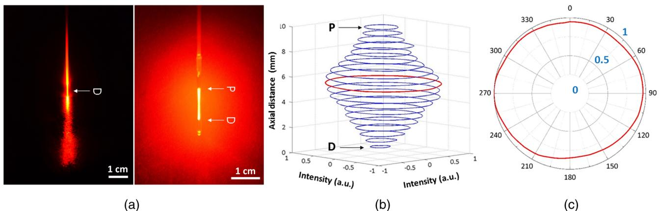
**Fig. 2** Spatial light distribution from diffusing applicator: (a) images of flat fiber (left) and diffusing applicator (right) with HeNe light transmission, (b) normalized 3-D distribution of light irradiation for diffusing applicator, and (c) corresponding polar emissions measured by goniometer (P = proximal and D = distal ends). Note that red color represents the maximum intensity used for normalization (5 mm from distal end).
