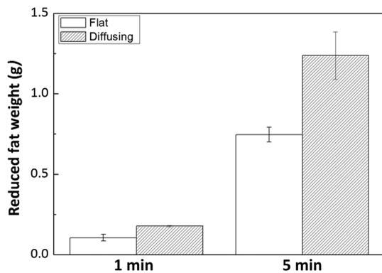
**Fig. 6** Comparison of tissue removal between flat fiber (10 W) and diffusing applicator (16 W) at two different irradiation times (1 and 5 min;  $N = 5$ ).
