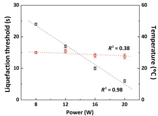
**Fig. 3** Liquefaction threshold and corresponding temperature as function of power with diffusing applicator.
