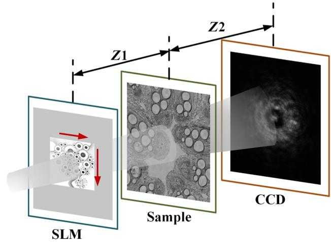
**Fig. 1** Schematic of the proposed method to record diffraction patterns.
