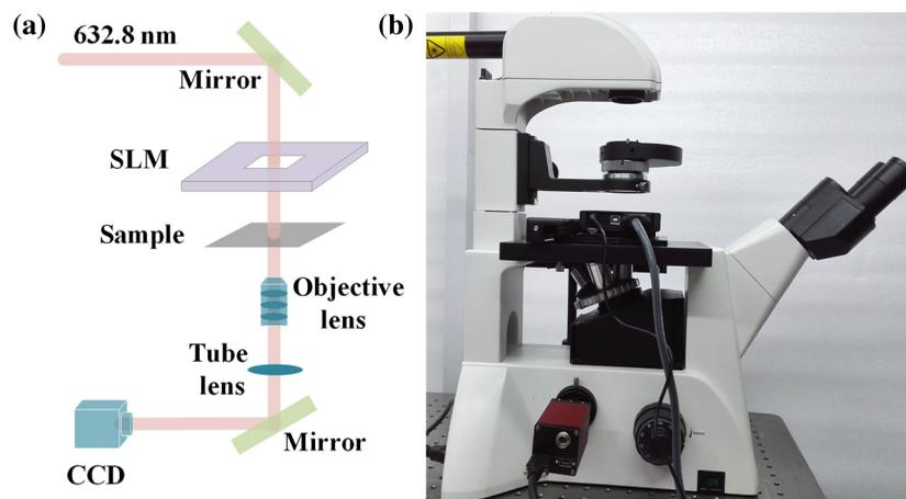
**Fig. 3** (a) Schematic and (b) actual device of the ptychography-based microscope integrated with SLM.
