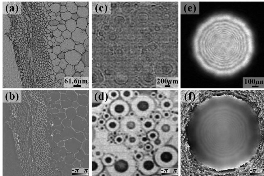
**Fig. 4** Reconstructed (a) modulus and (b) phase of the sample; (c) modulus and (d) phase of the transmission distribution of the SLM; (e) modulus and (f) phase of the incident beam on the SLM.
