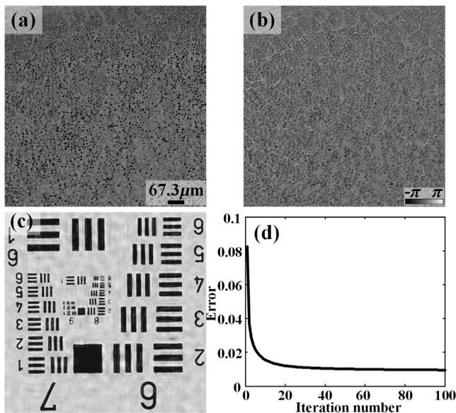
**Fig. 5** Reconstructed (a) modulus and (b) phase distribution of a slice of corn seed; (c) amplitude distribution obtained for a USAF 1951 resolution target; and (d) progression of the error over 100 iterations.
