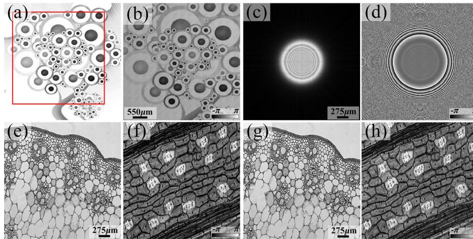
**Fig. 2** (a) Pattern loaded on the SLM (the red square indicates the illuminated section on the SLM); (b) reconstructed phase distribution of the SLM; reconstructed (c) amplitude and (d) phase of the incident beam on the SLM; (e) amplitude and (f) phase of the original object; reconstructed (g) amplitude and (h) phase of the object.
