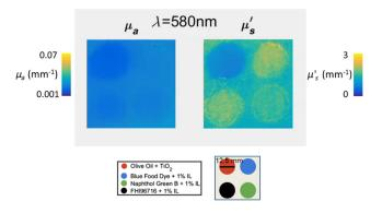
**Fig. 5** Spectral cube  $(x, y, \text{ and } \lambda)$  for absorption and reduced scattering coefficients of the multiwell phantom. Schematic representation of the wells with the silicone-based solid background is shown (Windows Media Player, 782 KB).
