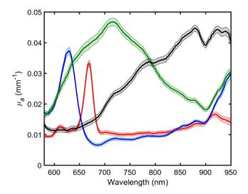
**Fig. 4** Plot of bulk  $\mu_a$  spectra for four solutions: three water-soluble dyes with 1% IL concentration. Olive oil is mixed with known concentration of TiO<sub>2</sub> (0.65 g/L). Each data point corresponds to the mean value of an optical property over a 6 mm × 6 mm ROI. About 208 data points in the 580- to 950-nm region are plotted for each concentration.
