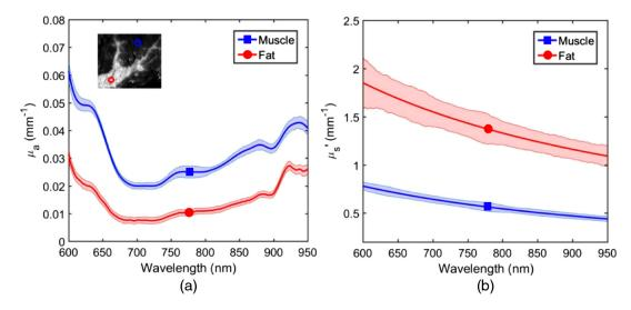
Fig. 6 Plot of (a) bulk  $\mu_a$  spectra and (b)  $\mu_s'$  spectra at two ROIs (3 mm  $\times$  3 mm): fat (red) and muscle (blue).
