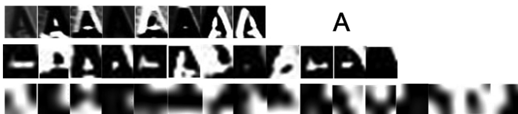
Fig. 12 An example of letter convolution results using the deep convolutional neural network. Top row: the first convolutional layer with eight feature maps. Middle row: 12 feature maps of the second convolutional layer. Bottom row: the third convolutional layer, which includes 16 feature maps.
