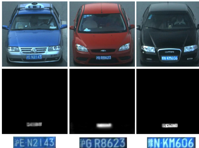
Fig. 7 Top row: three car images segmented from the traffic video. Middle row: corresponding saliency maps for license plates. Bottom row: detected license plates.
