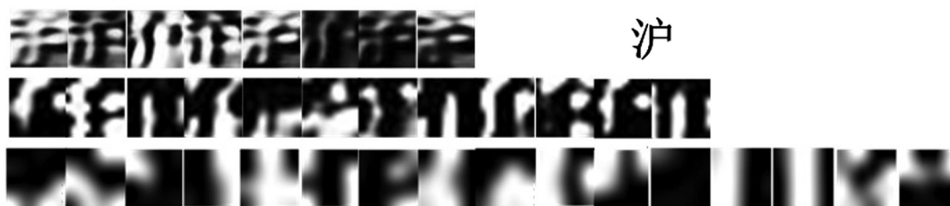
Fig. 11 An example of Chinese character convolution results using the deep convolutional neural network. Top row: the first convolutional layer with eight feature maps. Middle row: 12 feature maps of the second convolutional layer. Bottom row: the third convolutional layer, which includes 16 feature maps.
