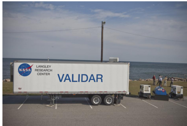
Fig. 2 The lidar is situated in a mobile trailer laboratory, parked at the Joint Expeditionary Base Little Creek, Fort Story to overlook the Atlantic Ocean and Chesapeake Bay. A beam scanner is attached to the roof for steering the lidar beam. (Photograph courtesy of: NASA/Sean Smith.)
