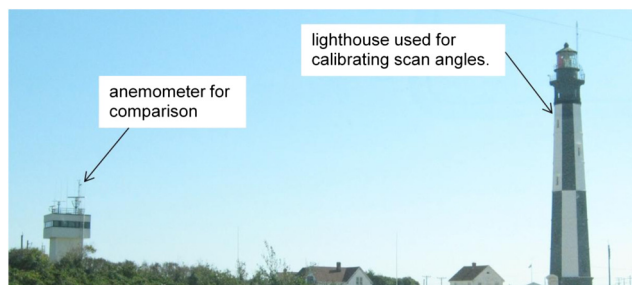
Fig. 3 The New Cape Henry Lighthouse provided a target for calibrating the lidar beam scanning angles. The lidar was scanned over an anemometer for comparison of the two sensors' wind measurements.
