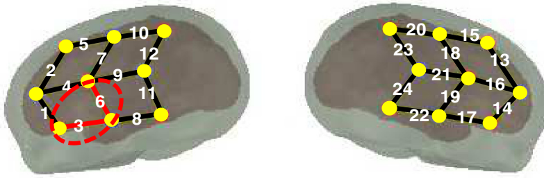
Fig. 1 Optode arrangement employed in the studies included 8 or 10 sources and 8 detectors, forming a total of 20 or 24 channels. The region of interest that we focused on is the left temporal lobe, formed by channels 3 and 6; it is highlighted in red.
