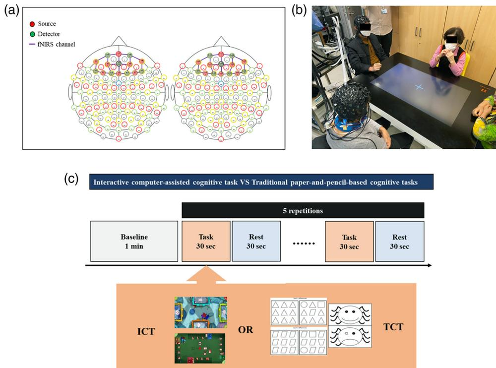
**Fig. 4** Experimental conditions: (a) the structure of the fNIRS channels, (b) measuring fNIRS hyperscanning data while subjects perform HAPPYTABLE<sup>®</sup>, and (c) experimental design and cognitive task paradigm.
