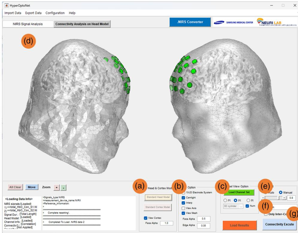
**Fig. 3** IBS step: (a) loading the head and cortex models, (b) viewing options of the head model, (c) section for loading the fNIRS channel set, (d) head model and synchrony display panel, (e) section for threshold selection, (f) selection of connectivity algorithms, and (g) the option for displaying only interbrain connectivity.
