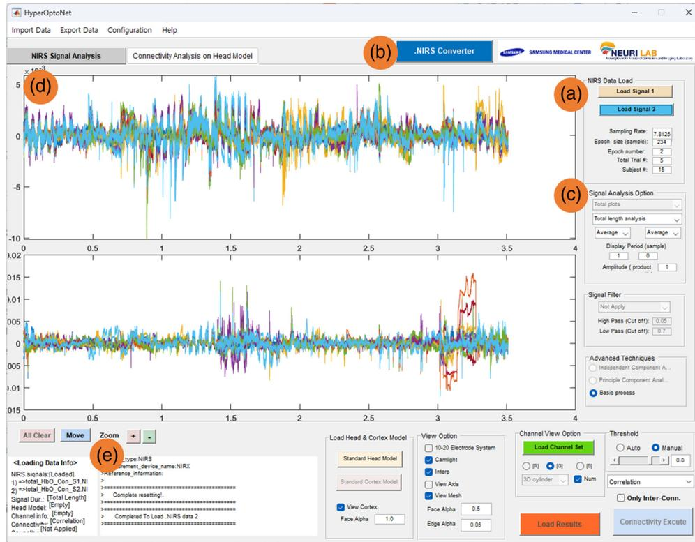
**Fig. 2** fNIRS hyperscanning data loading step: (a) “data load” section, (b) the button for loading.NIRS file converter, (c) “signal analysis” section, and (d) hyperscanning signal plotting panel, and (e) information panel.
