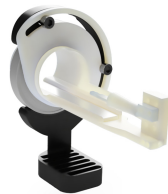
Fig. 9 Dedicated mouse positioning system. The system incorporates an anesthesia delivery mechanism and a bite bar. In addition, it allows for the positional adjustment of the mouse along two degrees of freedom: a translational one aligned with the bite bar and the mouse's spine, and a rotational one roughly about the mouse spine axis. This setup permits adjustments for a gimble configuration setting the pivot for the additional rotational degrees of freedom on or near the mouse right eye, using two additional rotational stages (not depicted). In turns, the setup was also placed on top of three motorized stages for the adjustment of the remaining translation degrees of freedoms along the X , Y , and Z axes.
