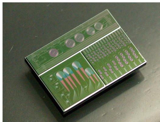
**Fig. 6** PIC sensor device with integrated photonics and electronics manufactured by the AIM Photonics teams.
