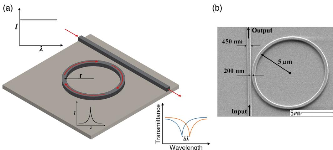
**Fig. 4** Ring-resonator sensor. (a) Schematic of a ring-resonator sensor. The linear waveguide provides input light to the loop waveguide at the coupling zone and captures output light from the loop for measurement. The presence of analyte will shift the resonance wavelength within the loop, which is detected in the output spectra, adapted from Ref. 10. (b) Micrograph of a fabricated ring resonator, adapted from Ref. 22.
