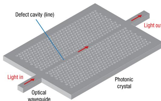
**Fig. 5** A 2-D PhC waveguide adapted from Ref. 30. The top and bottom milled areas form a PhC with a photonic bandgap. Light is confined to defects which, here, is the region absent of holes, which forms the central waveguide. Introducing analytes near the PhC changes the RI and the cutoff frequencies of the bandgap.
