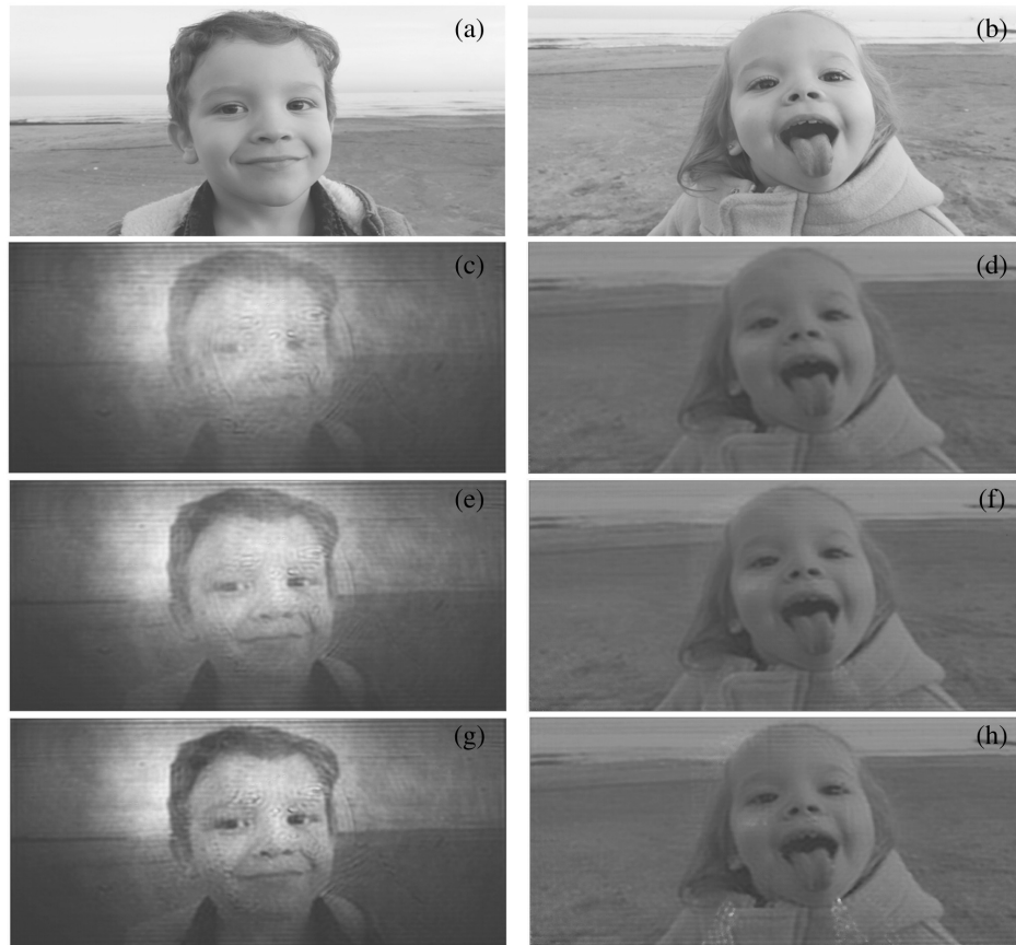
Fig. 5 (a) Target amplitude and (b) phase images, and (c), (e), and (g) corresponding amplitude and (d), (f), and (h) phase images recorded for sampling gratings of 1 \times 1 , 2 \times 2 , and 5 \times 5 pixels/cell, respectively.
