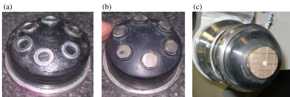
Fig. 8 “Grolishing” tool. (a) Stainless steel ring. (b) Diamond pill tablets. (c) Brass ingot.
