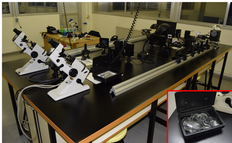
Fig. 12 Optical tables where the students perform the experiment. The different materials that the students have are optical bench, lensmeters, sets of convergent and divergent lenses to characterize (see the red box on the bottom-right corner of the image), and different supports for lenses and other auxiliary material (e.g., screens, transparencies, lamps, and diaphragms).
