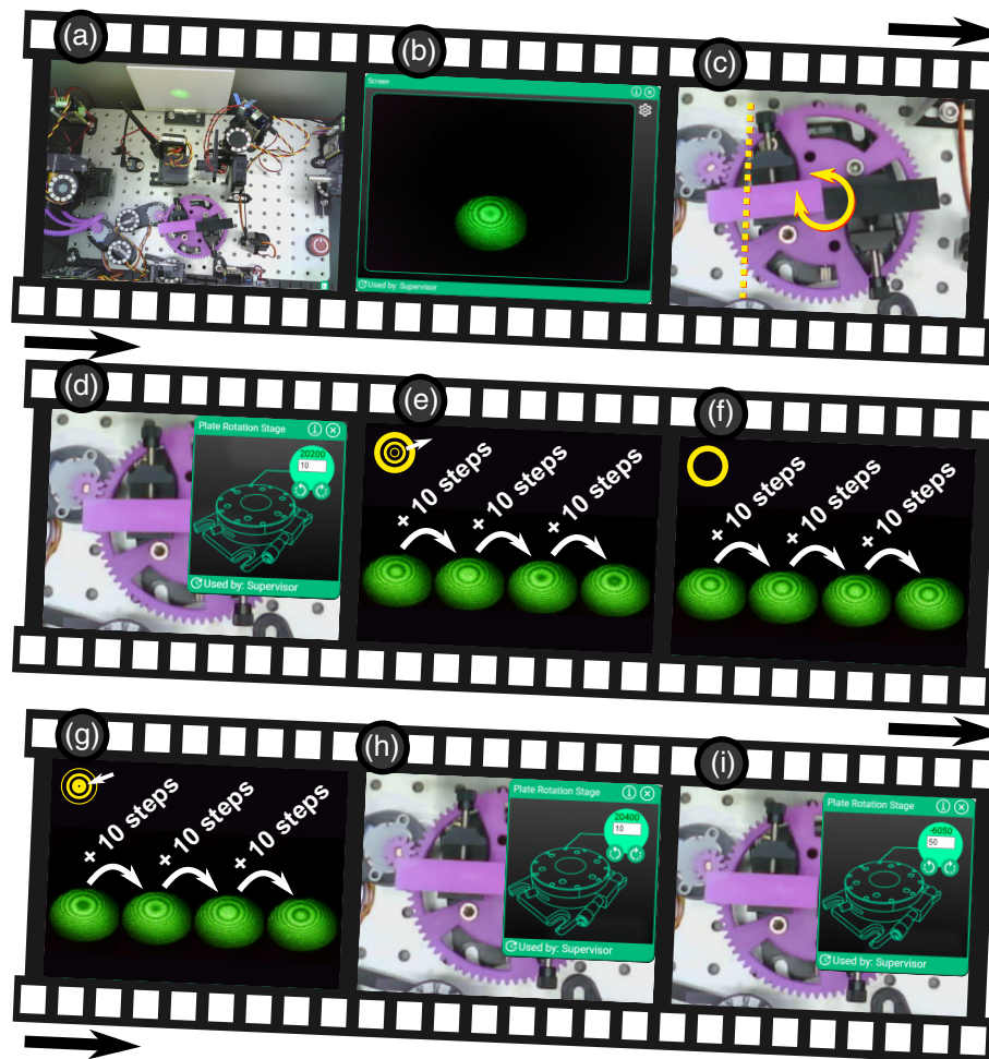
Fig. 9 Sequential illustration of the workflow of the experimental task “adjust the acrylic glass plate such that it stands perpendicular to the beam path” carried out by a student. (a) View given by the overview cam (Table 1 item III), (b) view given by the screen (Table 1 item 7), (c) detail of the overview with beam path indicated as a dashed line, (d), (h), (i) detail of the overview with component control window, (e)–(g) consecutive views shown from the screen. A description of the sequences is given in the text.
