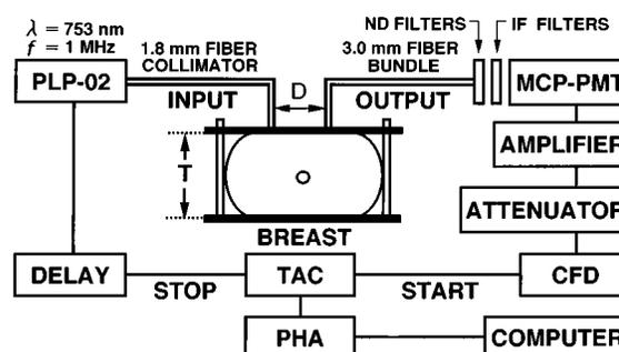
**Fig. 1** Block diagram of the apparatus for measuring optical parameters in the breast. PLP, picosecond light pulser; MCP-PMT, microchannel plate photomultiplier tube; CFD, constant fraction discriminator; TAC, time to amplitude converter; PHA, pulse height analyzer.
