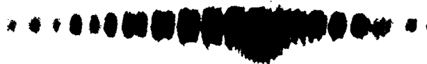
Fig. 6 Interference pattern produced by focusing an He:Ne laser through a 25 \mu\text{m} capillary.
