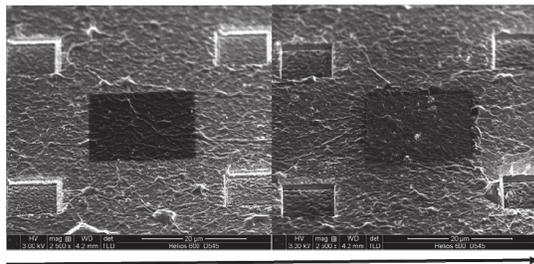
Figure 1. SEM images of the effect of increasing fluence on the GO sample there is an immediate change in contrast initially but it is clear that at higher fluences the surface undergoes significant damage.
