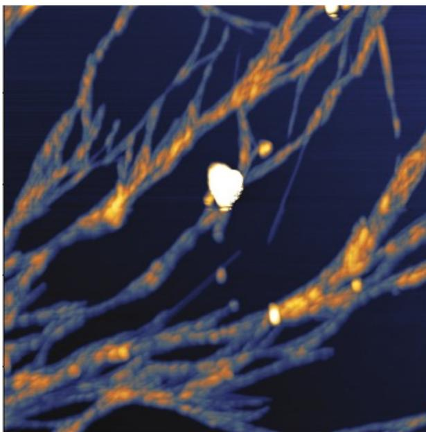
Figure 1 ac-βLβIβA on mica surface, imaged by AFM. The scale is 10 μm. The peptide was dissolved in methanol and mixed with isopropanol for deposition. Typical heights of fibres are 20-30 nm
