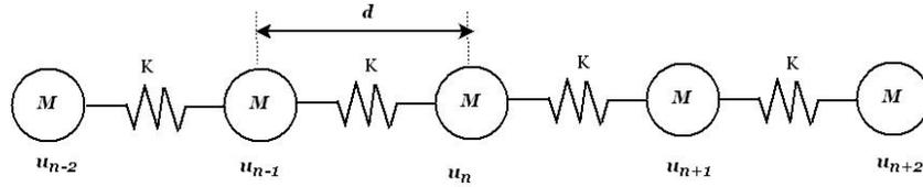
Figure 3. 1-D discrete lattice model
