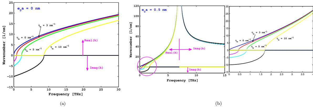
Figure 8. Wavenumber dispersion in monolayer Graphene sheets (a) local elasticity ( $e_0a = 0 \text{ nm}$ ) (b) Nonlocal elasticity ( $e_0a = 0.5 \text{ nm}$ ). Wavenumber variation at lower frequencies is shown separately for clear visibility
