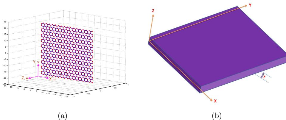
Figure 7. Single-layered Graphene sheet: (a) Discrete model (a monolayer Graphene of  $40 \times 40$ , consists of 680 carbon atoms arranged in hexagonal array) (b) Equivalent continuum model.
