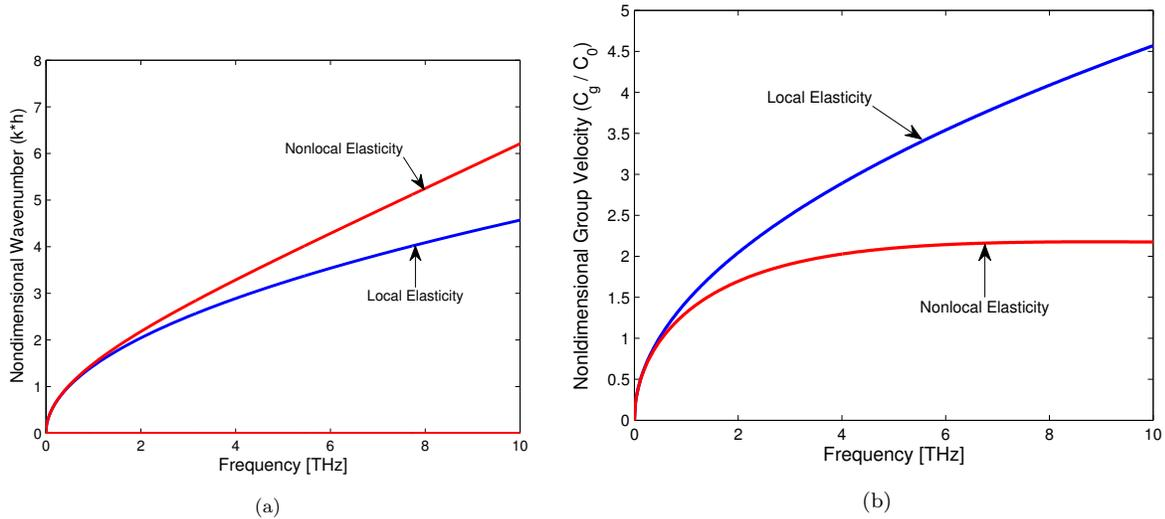
Figure 6. Wavenumber and dispersion relations for Stress gradient Nano beams
