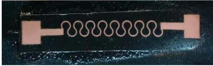
Figure 3. A stretchable interconnect for wearable electronics fabricated using a new stamping process with PDMS integrated directly into the fabric substrate.
