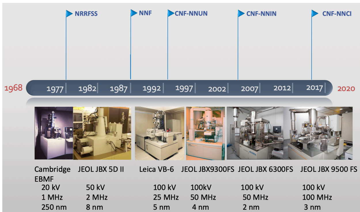
Figure 7. Timeline showing the parallel between the evolution of the shared user facility networks and the acquisition of advanced electron beam lithography tools.
