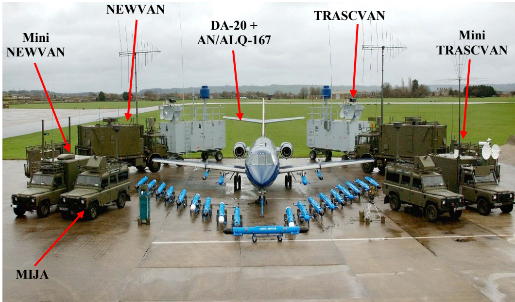
Figure 1. Examples platforms used to generate jamming: Mini NEWVAN, NEWVAN, Mini TRASCVAN (TV), TRASCVAN, MIJA, AN/ALQ-167 [1]
