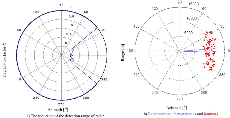
Figure 3. "Ideal" radar disturbed by 4 low-power interference transmitters' packages.
