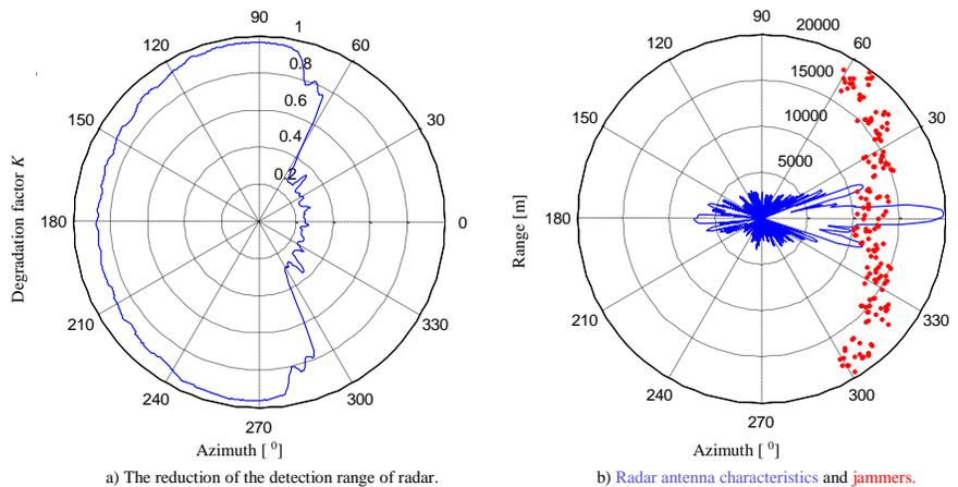
Figure 6. Typical radar disturbed by 4 low-power interference transmitters' packages.
