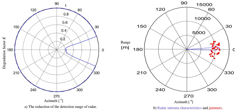
Figure 1. "Ideal" radar disturbed by 2 low-power interference transmitters' packages.
