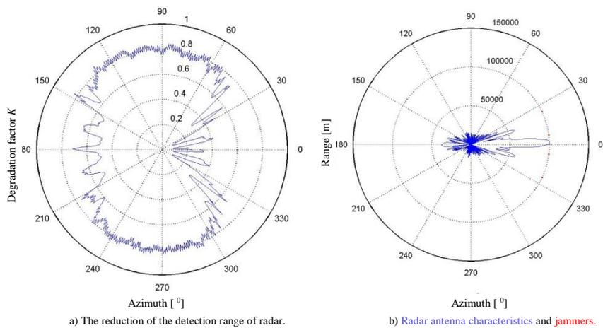
Figure 5. Typical radar disturbed by 4 high-power interference transmitters on the aircraft.
