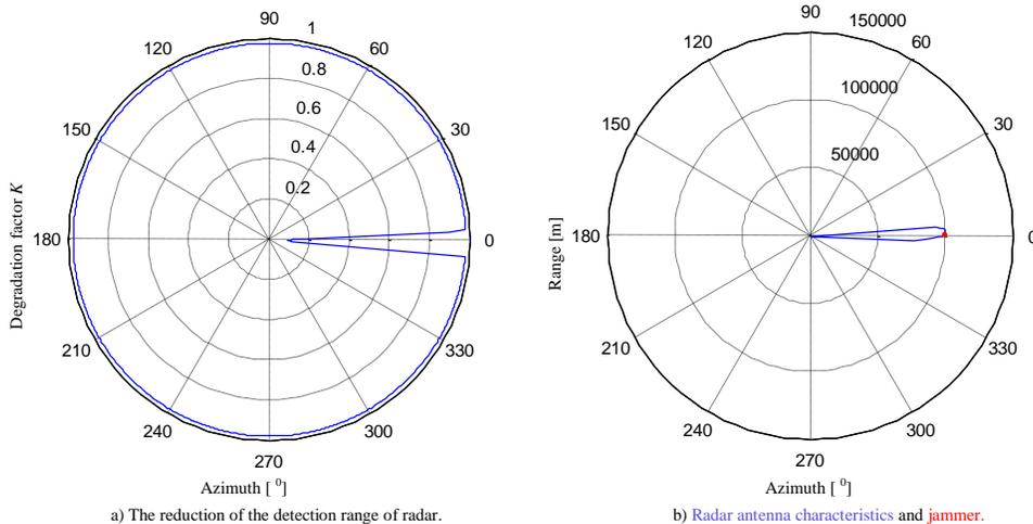
Figure 2. "Ideal" radar disturbed by 1 high-power interference transmitter on the aircraft.
