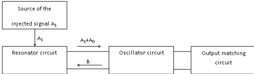
Figure 7. General block diagram of the injection synchronized oscillator.
