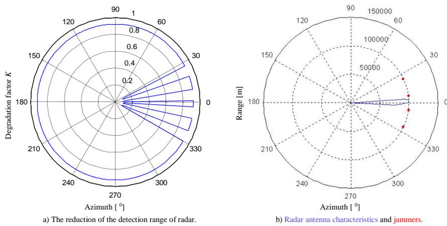
Figure 4. "Ideal" radar disturbed by 4 high-power interference transmitters on the aircraft.
