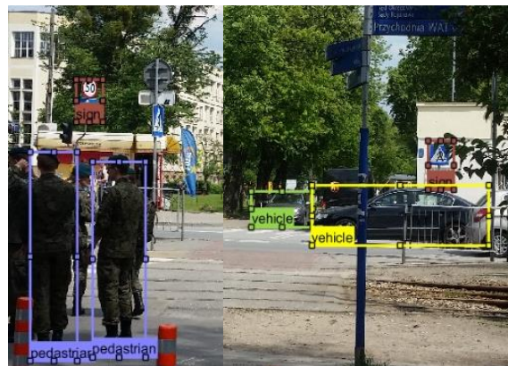
Figure 14. The result of pedestrians, vehicles and road signs recognition with using the neural network
