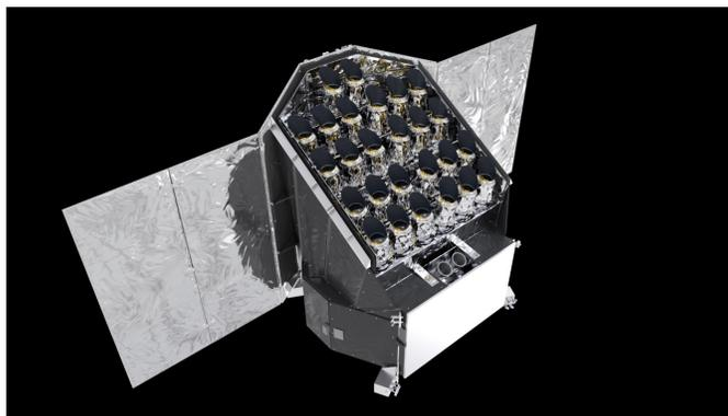
Figure 1. Artist impression of the PLATO Spacecraft with the 26 camera visible. The Electronic Units are hidden behind the radiator visible in front below the cameras. Credits: OHB System AG
