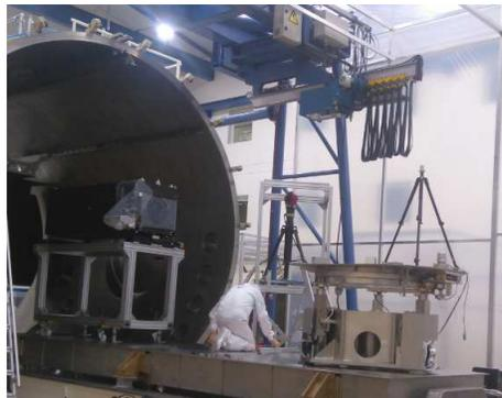
Figure 5. Stray-light measurement facility preparation – collimator (left) – rotating stage for the instrument (right)
