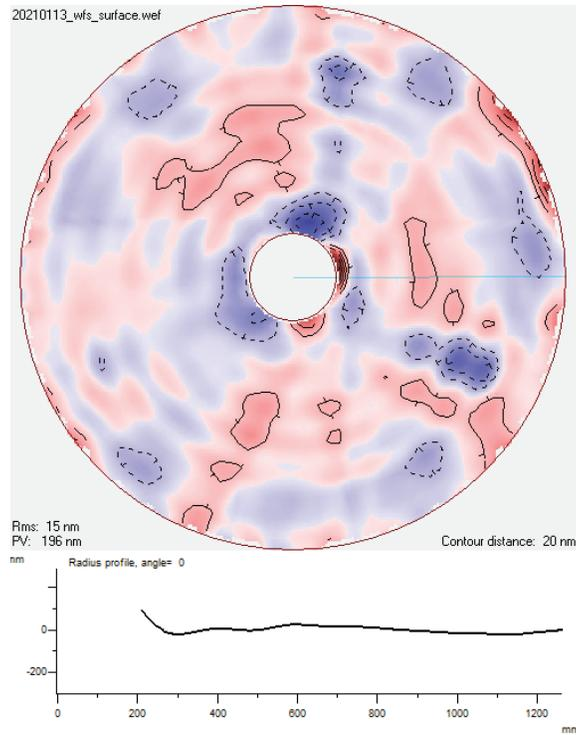
Figure 7. Latest surface accuracy measurement performed at OPTEON.
