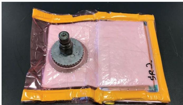
Figure 2. Sample in the vacuum bag before curing.
