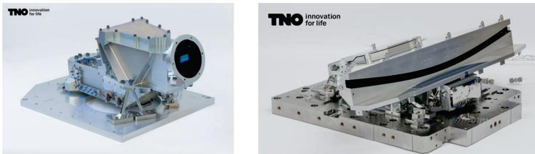
Figure 1. Picture of UV1 spectrometer (left) and TSBOA (right) PFM model. Picture credit TNO.
