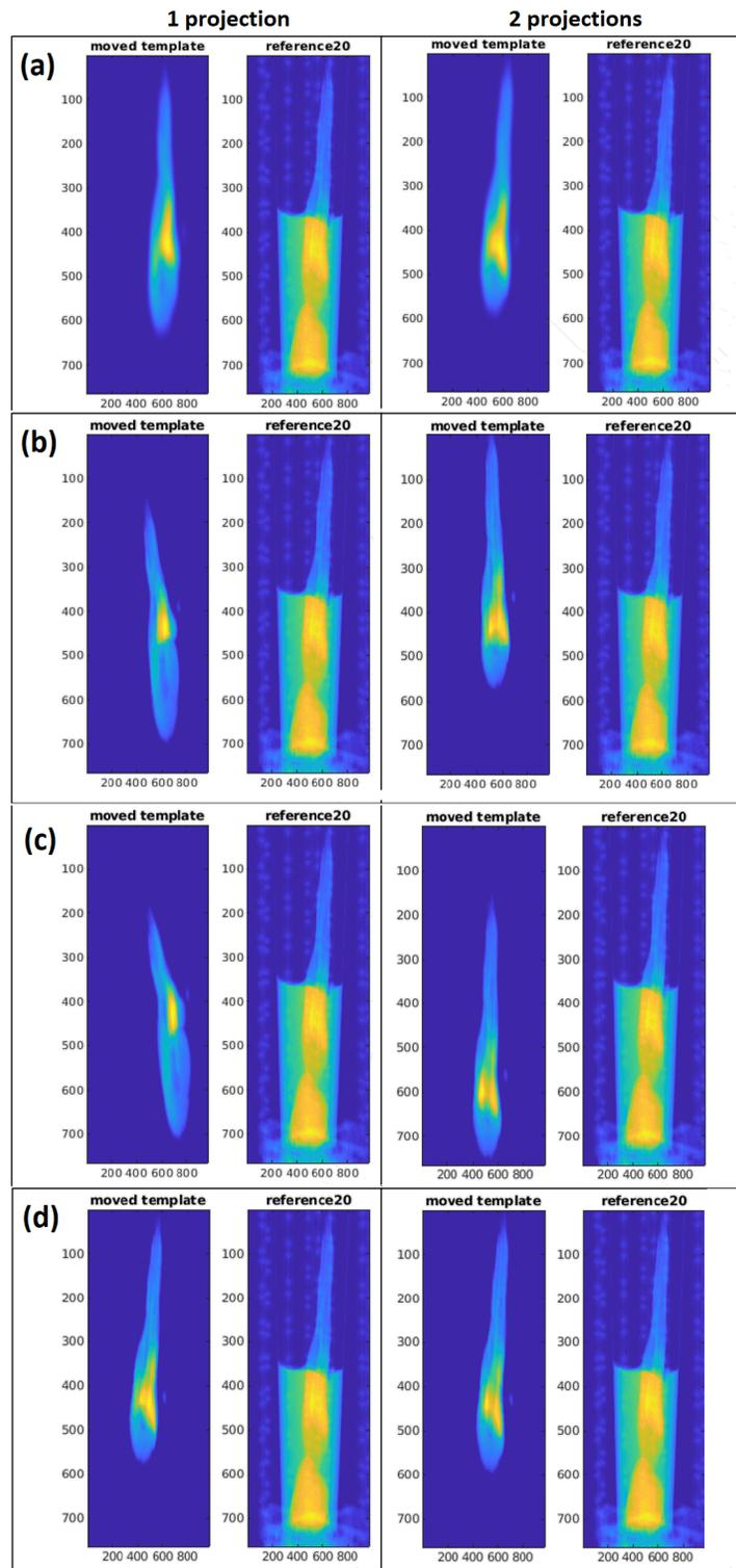
Figure 4. Demonstration of the four different setups. Registration performed with 1 projection at angle  $45^\circ$  (Left) and with 2 projections at angles  $0^\circ$  and  $90^\circ$  (Right). Rows (a) to (d) correspond to registration results for frame 20 for setups 1 to 4 respectively.
