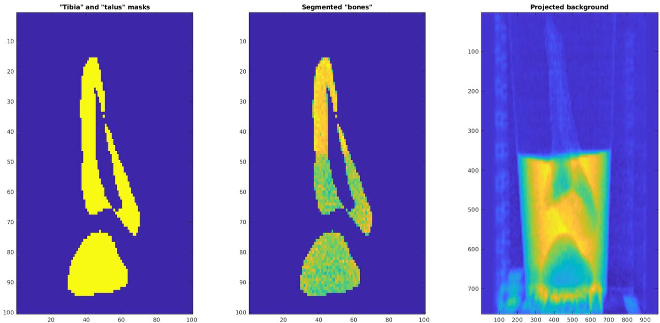
Figure 2. Demonstration of data pre-processing. *Left*: A slice through the bone masks volume, top:  $m_{tibia}$ , bottom:  $m_{talus}$ ; *Middle*: A slice through the segmented bones volume  $s_{bones}$  acquired by applying the bone masks to the full reconstruction of the initial pose; *Right*: A simulated projection of the "background",  $g_{bg}$ .
